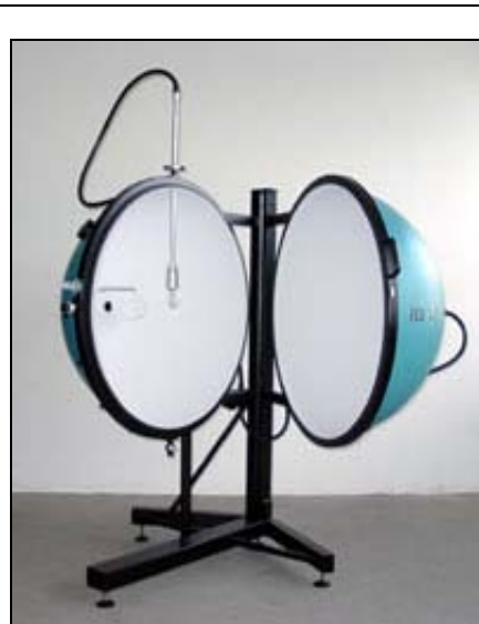
Diagram 1: example of a typical integrating sphere
